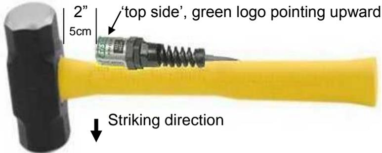
Mount the trigger switch on the top side of the hammer handle about two inches back from the head. Use electrical tape to fasten switch and cable securely. The 'top side' label and green GISCO logo should be pointing upward.
